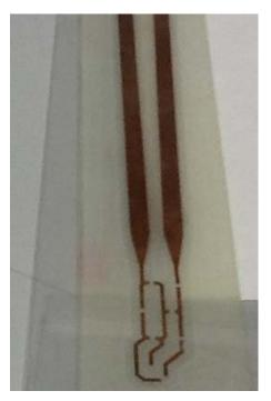
The photograph shows co-planar strip lines on a printed circuit board. All other metallization – top and bottom – has been scraped away to reveal a bare fiberglass resin dielectric. The circuit traces at the bottom are for implementing a discrete component *balun* – a device for converting and matching a change in transmission line topologies.
